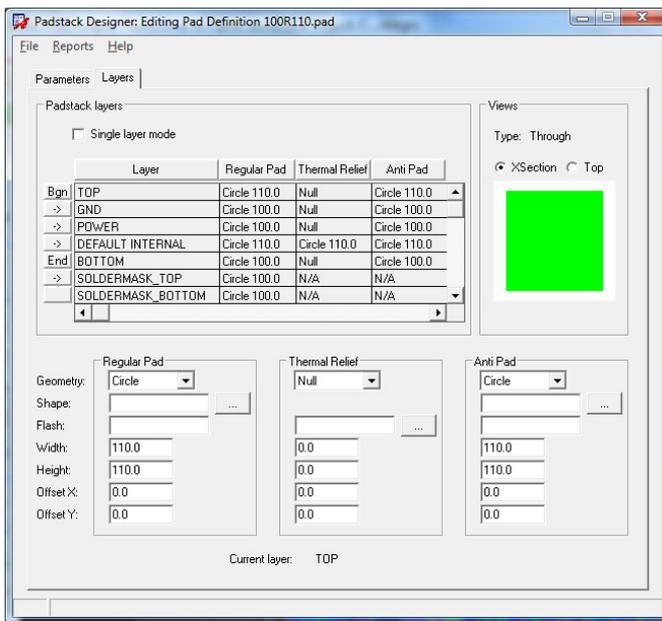
For this specific pad, the drill and the pad are both set 110, then intention being to remove the pad. A better practice would be to set the pad to be smaller than the drill to ensure that there were no small remnants of the pad after drilling, as such, left-click in the TOP (layer) cell, set the Regular Pad to, say, 80 and set the Thermal Relief and Anti-Pad to “null” as shown.
